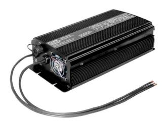
**K-LINE** DP4-24/30 consists of a switched mode DC power supply unit and a DC/DC voltage regulator for the back-up battery. If it is used together with a battery charger and a battery pack, under normal conditions, the DC output is supplied from the switched mode power supply unit. In case of AC failure, the DC output is then supplied from the back-up battery via the DC/DC voltage regulator, thus forming an uninterrupted DC power supply system.
